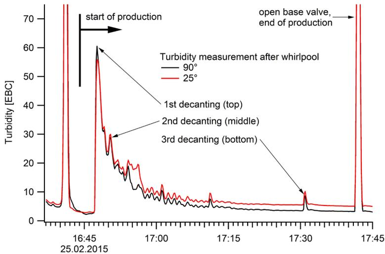
**Process of hot break separation at the measuring point after the whirlpool**
