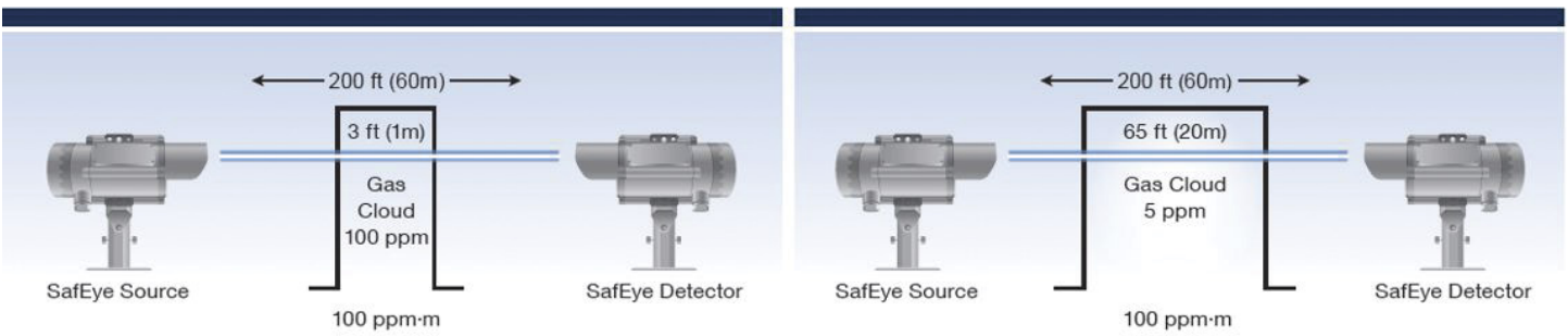
100 ppm-m = a cloud of 100 ppm methane gas that is 3 ft (1m) wide
