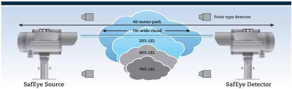
This scenario shows how the matrix of point type detectors can miss a leak or eventually only see diluted gas levels whereas SafEye 900 Open-Path will, in this case, measure 20% LEL x 7m = 1.4 LEL, m - well above 1 + LEL and 1 + LEL above 1 + LEL and 1 + LEL above 1 + LEL above 1 + LEL and 1 + LEL above 1 + LEL above
