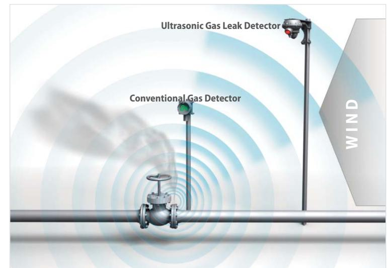
Ultrasonic gas leak detectors do not need physical contact with the gas. They are unaffected by wind, gas dilution, and the direction of the gas plume.
