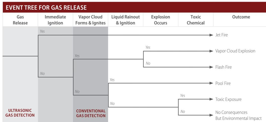
The gas release event tree illustrates the sequence of events that can take place in the event of a gas release. The figure shows that UGLD responds at gas leak initiation whereas conventional detectors only respond when the gas has accumulated and formed a vapor cloud.
