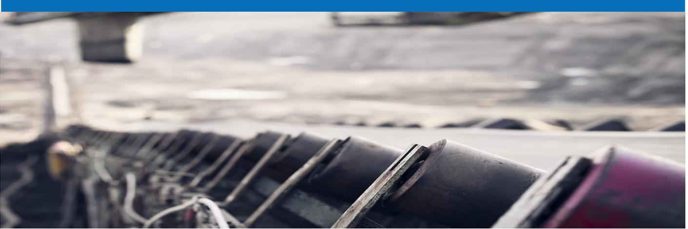
**Fires on conveyor belt systems are commonly caused by the friction of the belt on seized idlers and rollers or from bearings overheating. In addition the product being transported may already be on fire. The situation becomes even more dangerous because a conveyor belt has the ability to spread a fire over long distances. Linesense digital Linear Heat Detection (LHD) offers a cost effective fire detection solution.**
