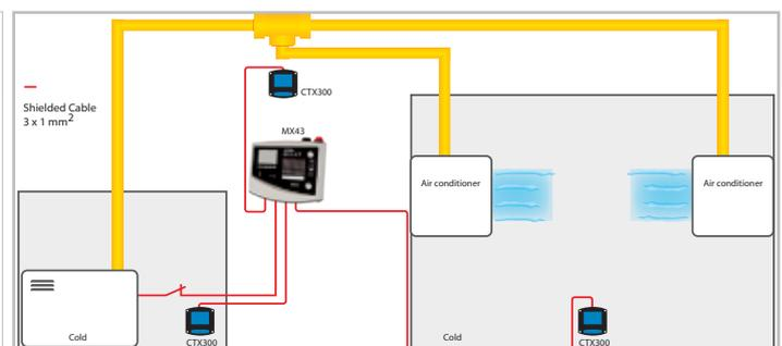
The sensors are placed near the ground level (because of the Freon density) usually in the engine room or technical room.
