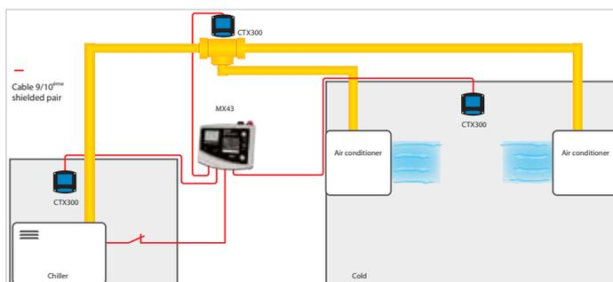
The sensors must be placed at a high level, usually in the attic, in order to protect people (engine room, technical room).
