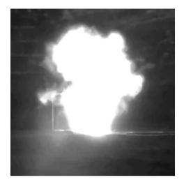
The image to the left shows a hydrogen explosion in near-infrared. The hydrogen fire is easily seen on the video.
