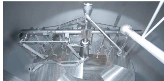
Picture 2: Lauter tun with raking device
